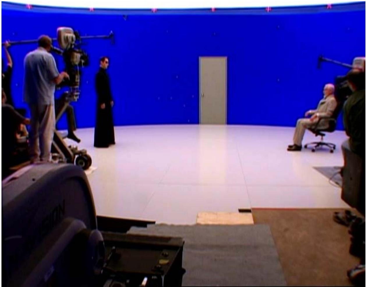
MATRIX RELOADED - Twin-Booms to cover A and B cameras (both on matching tight shots) Note the similar relative-distances from speakers mouths.
