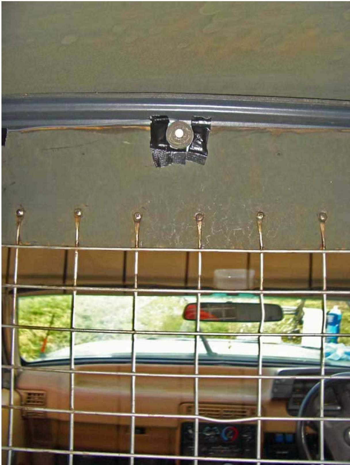
a Sanken CUB-01 Boundary layer Microphone - to capture the dialog of a character in the back of the vehicle, during a stunt - this is attached to the remote "C" car.
