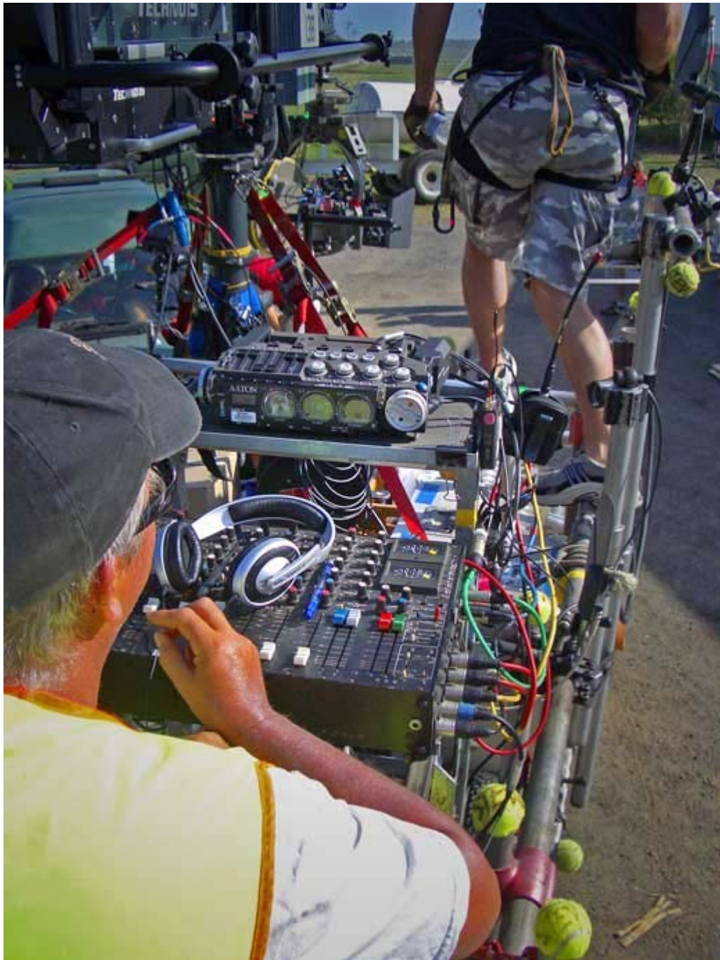
Guntis' Trolley on the towing vehicle. You can see the aaton Hard-disk recorder on top, and his Cooper 108 Mixing panel under the headphones.
